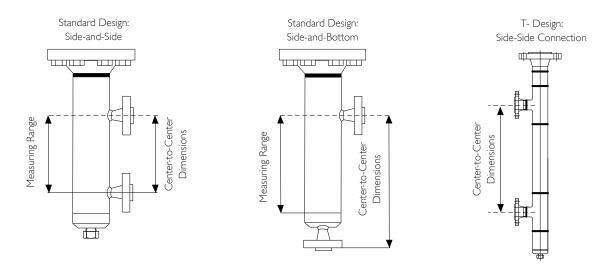
This configuration allows an instrument to be isolated with valves for maintenance without disturbing plant operation. It is also useful for in-tank restrictions that do not allow mounting of the instrument in a vessel. This approach offers many advantages when solving application challenges. The instrument is mounted on top of the chamber with the flanged or threaded instrument connection. A thread version is available for the vertical float level switch.
