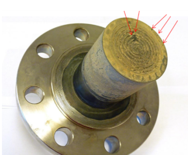
Figure 3 & 4: Within one year the Tantalum diaphragm is severely damaged due to loss of corrosion resistance due to welding.
