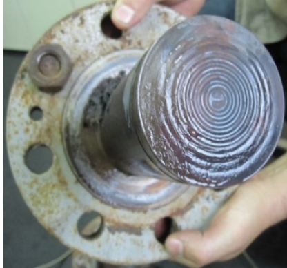
Figure 2: 316 Stainless Steel diaphragm severely damaged within the first year operation.
